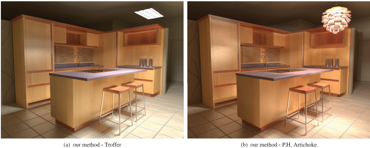
Fig. 16. A luminaire can have a substantial effect on the appearance of the interior design. Each image shows the same kitchen room rendered with a single luminaire as the only light source using our method, including global illumination. Notice how the shadows cast by the stools and the highlights on the left cabinet mirror the structure of each luminaire.
