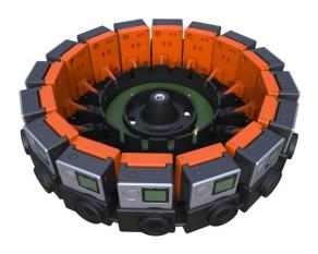
Googe's Jump 16-camera rig (there are other competitive devices) simultaneously captures 360 degree scenery. Images from each camera can be stitched together to create dynamic backgrounds for virtual and augmented reality systems.
