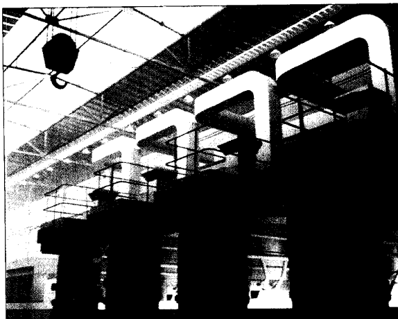
“Simulated Steel Mill” by Stuart Feldman and John Wallace (Program of Computer Graphics, Cornell University, 1987) was created using a modified version of the hemicube radiosity algorithm, computed on a VAX 8700, and displayed on a Hewlett-Packard Renaissance Display. The environment consists of approximately 2,000 patches and 55,000 elements and was one of the more complex environments computed to date.
