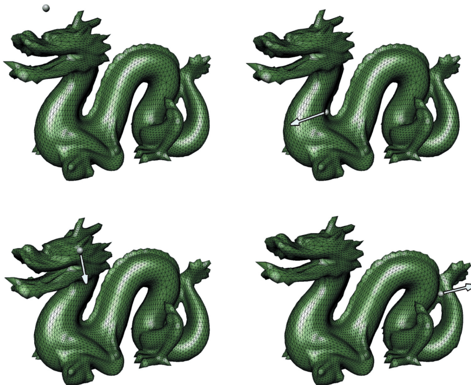
Fig. 22. Deformed dragon model ( L = 3 ) shown in a force feedback simulation, contacted by a small white ball (force direction indicated by arrow). The undeformed model is shown in the top left image, and other images illustrate hierarchical GF deformations due to forces resolved on constraint level 0. This very large model compresses extremely well (approx. factor of 100 at 5% RMS error) and is therefore suitable for interactive force feedback simulation.
