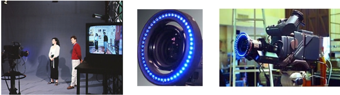
Figure 3.11: The BBC's LiteRing system uses low-powered, colored LEDs to illuminate a mesh screen, which then feeds a traditional linear keying process. The integral part of the system is the gray mesh, which is made up of millions of very small glass beads. These beads make the screen highly retroreflective, allowing it to reflect almost all incident light back to its source, independent of the angle of incidence to the screen. This retroreflectivity cause the background to take on the color of the LEDs, observable only from the lens' location. Images courtesy of Reflecmidia.
