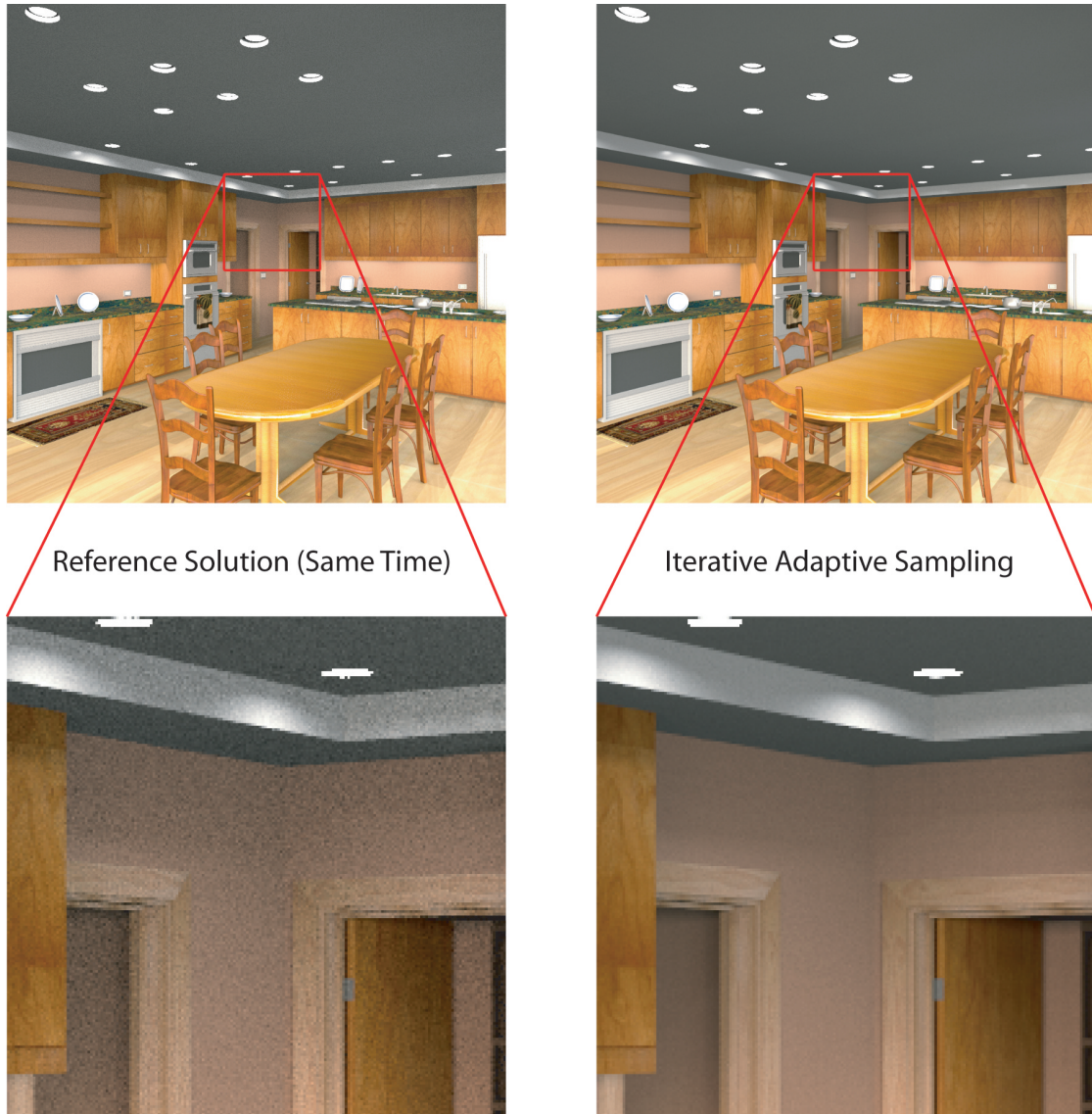
Figure 4.7: Kitchen with Environment Lighting Qualitative Comparison. The bottom row contains closeups showing the effectiveness of our algorithm when rendering scenes with direct illumination from environment maps.
