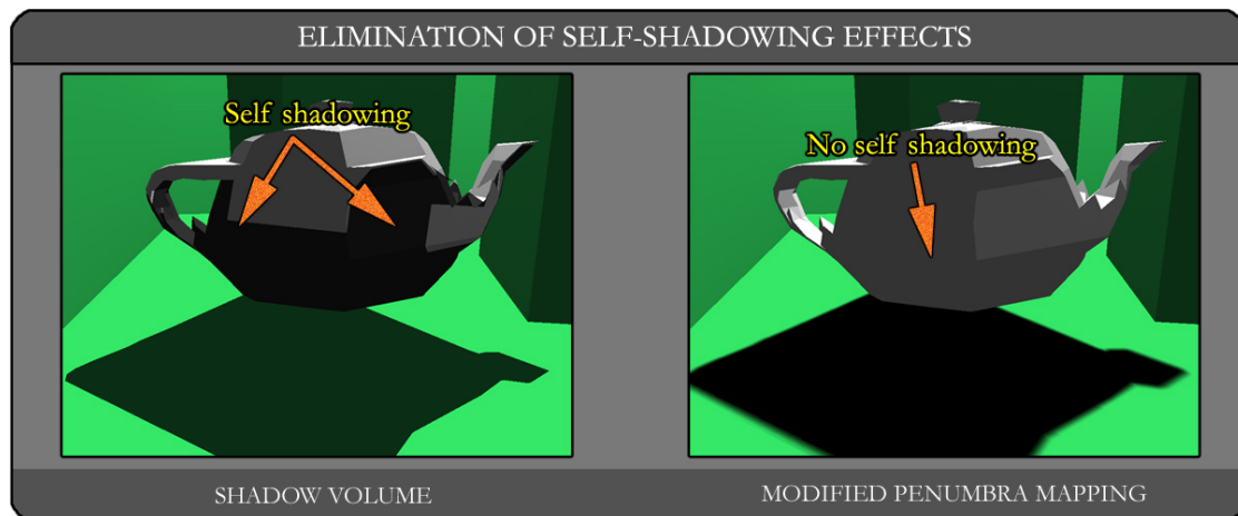
Figure 5.10: The figure above compares the output of an algorithm that generates self-shadowing effects and our approach, which does not.
