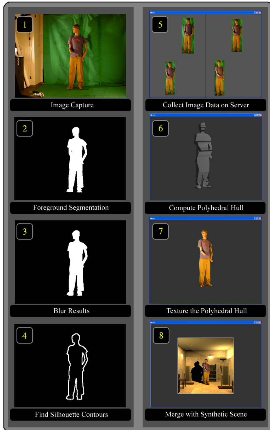
Figure 3.1: The diagram above depicts each stage of the image processing, geometric reconstruction and compositing process.
