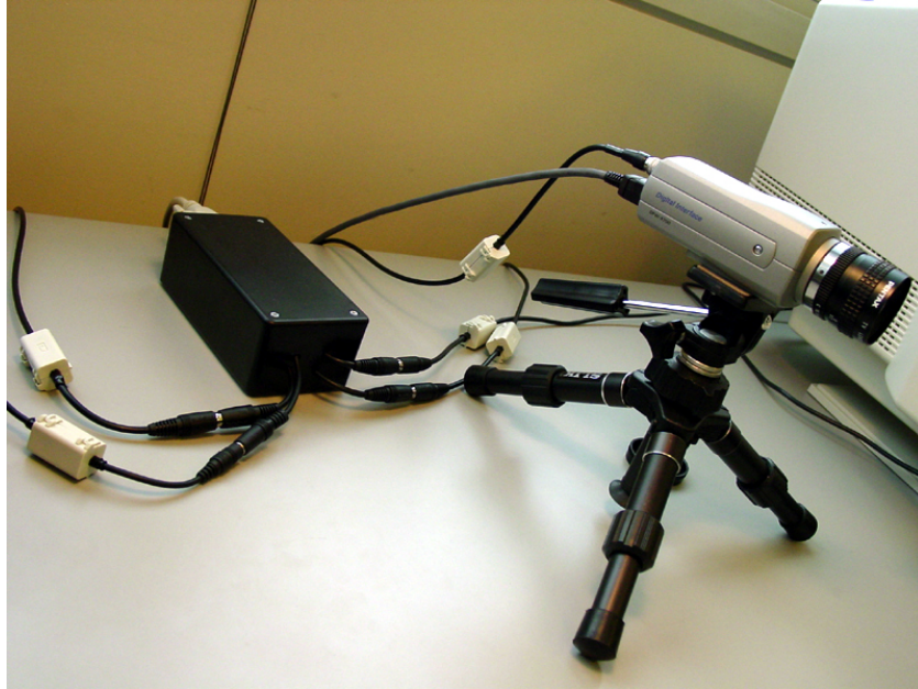
Figure 3.3: The image above shows a DFW-X700 camera and the trigger circuit box.
