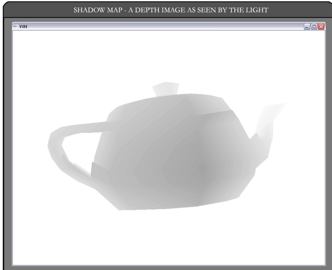
Figure 5.1: In the figure above, a teapot has been rendered from the point of view of the scene's light. By using intensity values to represent distance, the figure shows the generated depth image (shadow map), which will be used during shadow computation. Darker regions of the image represent smaller depth values, where the object is closer to the camera. Conversely, lighter areas indicate larger depth values where the object is a greater distance from the camera.
