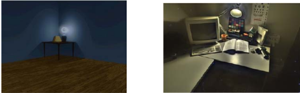
Figure 2.1: Two images illustrating halo artifacts. The image on the right is output from Pattanaik's multi-scale model of adaptation [Pattanaik98]. On the left is output from Chiu [Chiu93]. Both suffer from halo artifacts around the light sources.
