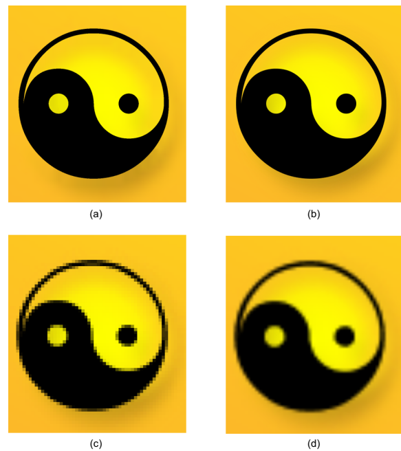
Figure 8: Reconstruction of lower left corner of yin yang example using (a) vector-based SVG rendering; (b) 230×256 FBT; (c) 460×512 texture map with nearest neighbor sampling; (d) 460×512 texture map with bilinear interpolation.
