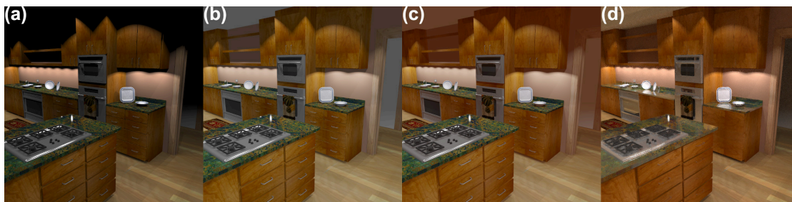
Figure 4.9: (a) Direct illumination, (b) contrast equalized version, (c) contrast equalized using hue shifted albedo image, and (d), full global illumination solution. Notice the hue differences between (a,b) and (d), and the similarity of (c) and (d).
