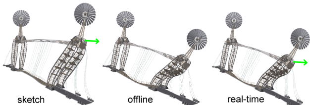
Figure 9: Basis from Sketch: (Left) User interacts with a linear model. Resulting shape is distorted. (Center) Applied force is recorded and sent to an unreduced offline static solver to solve for the corresponding nonlinear shape. Several such shapes are then processed by mass-PCA to obtain a basis of motion. (Right) If same force is re-applied during the reduced runtime simulation, a shape which is visually almost indistinguishable from the center image emerges.
