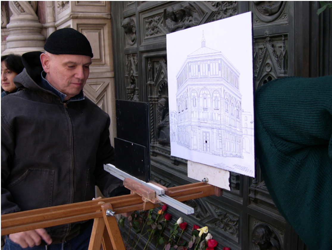
Figure 2.4: A recreation of Brunelleschi's experiment at the entrance to the Duomo in Florence facing the piazza and baptistry. A perspective image (reflected in a mirror) of the baptistry is seen through a small hole in the board. Correct placement of the image and mirror make it possible for the perspective image to exactly replace what the viewer would see if the mirror were removed.
