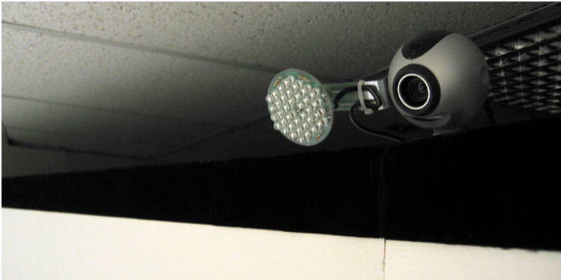
Figure 4.2: An image of one of the two cameras used to track users within a specified area. Each camera was paired with an array of infrared LED’s that was aimed and targeted to match the camera’s field of view.
