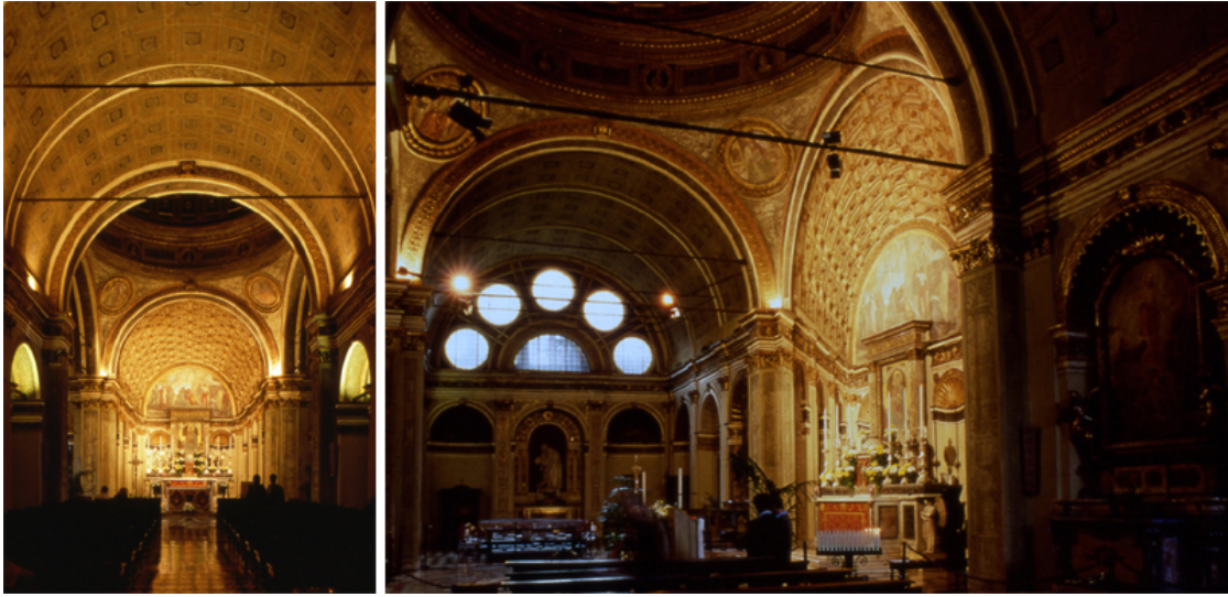
Figure 2.17: Comparison of an on-axis view ( left ) and an off-axis view ( right ) demonstrate the use of a compressed, perspective transformed geometry to give the impression of a deeper apse than could actually have been constructed under the space constraints. When viewed from the nave the illusion is plausible, but an off-axis view reveals that the apse is only a meter or two in depth.
