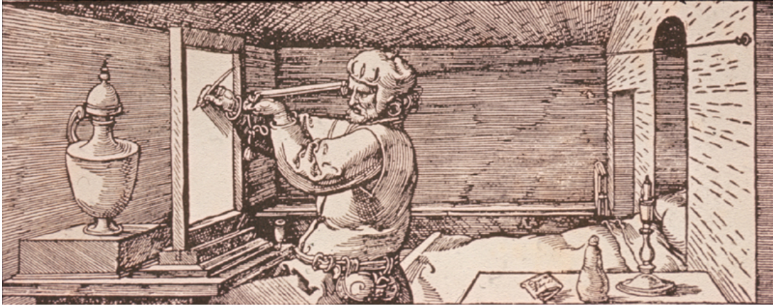
Figure 2.7: A second machine for the construction of perspective images by Albrecht Dürer. This version replaces the hinged opaque plane with one that is fixed and transparent. While the artist sits close to the transparent plane, the eye position or station point is where the string is fixed to the wall.
