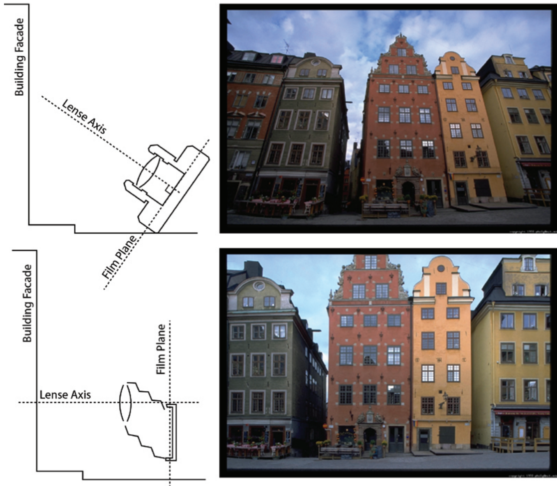
Figure 3.5: A comparison of two types of cameras typically used for architectural photography demonstrate the difference between a standard viewing camera (top) and a skew camera (bottom). The skew camera is often considered ideal for photographing architecture because the image plane can be aligned with a major facade independent of the direction of view - which in this case is angled upward in order to encompass the entire scene.
