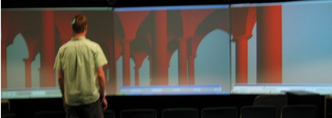
Figure 4.10: Three displays tile to form a single wide angle perspective image. The image is updated based on the viewer's location. Note that in this figure, the width of the equally sized columns look wrong since the real camera used to take this picture is in the wrong location. However, from the viewer's point of view the geometry appears correct (Figure 4.11).
