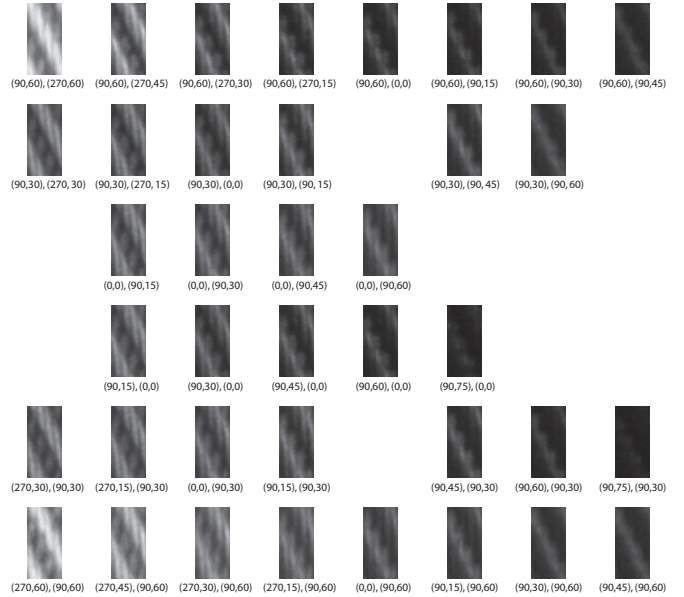
Figure 6: Measurement images grouped in columns based on their half vector. Two pairs of numbers under the images are the incident and exitant directions. Note the similarity of the images in a column.
