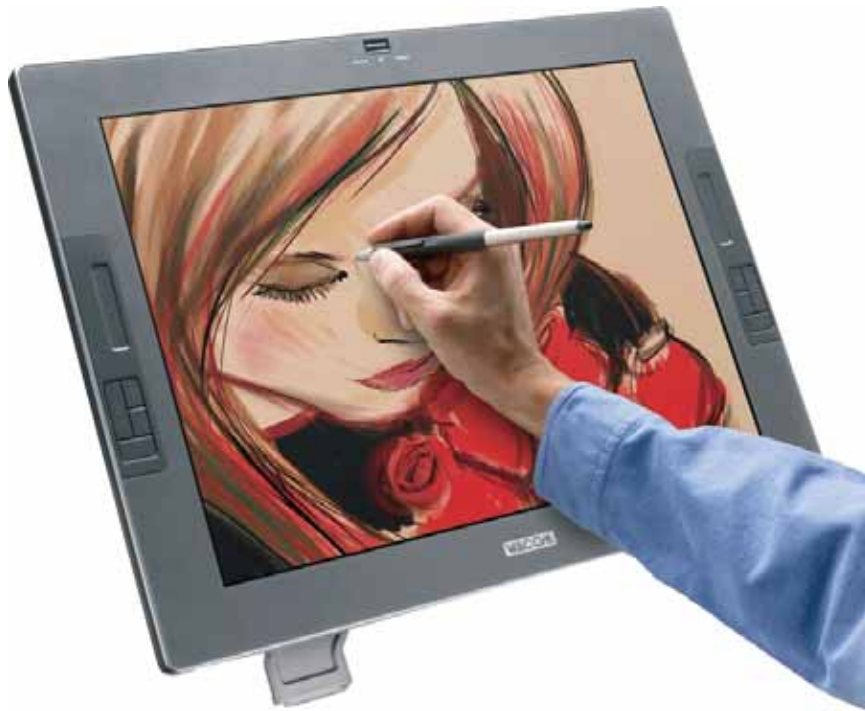
Figure 4.20: Tablets with built-in displays, such as the WACOM Cintiq, give users direct feedback and most closely simulate the experience of using a pencil. [Cin].
