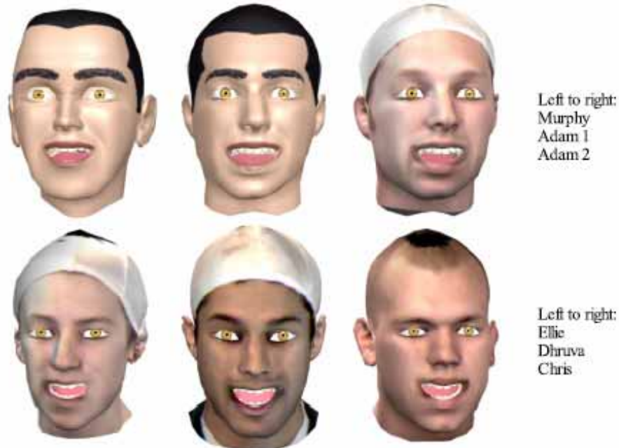
Figure 4.5: Four fitted scans posed in the same facial expression using the prototype rig. The top left face is the prototype, Murphy. The top middle is the same face as the top right, with Murphy’s generic texture in place of the scanned texture.[Bib04]
