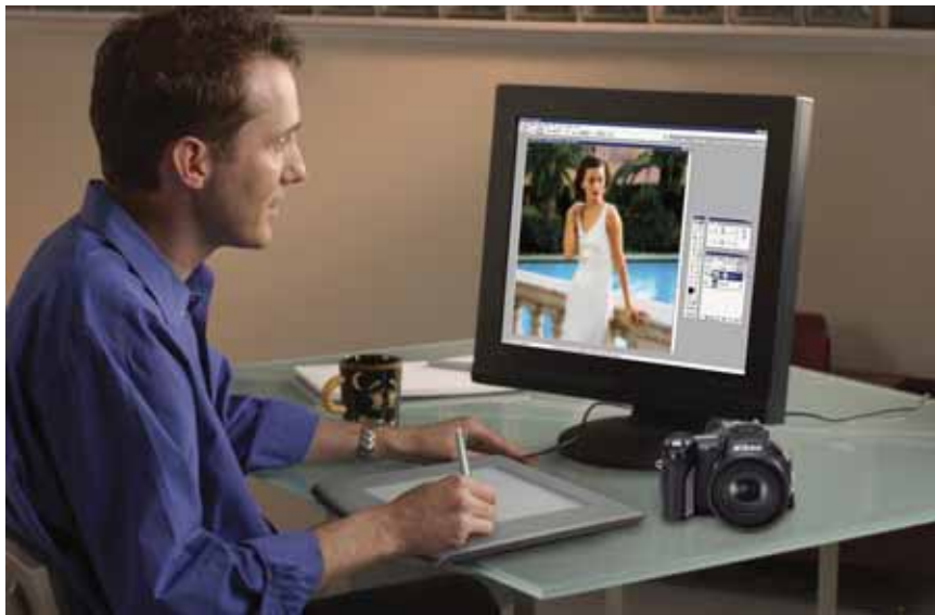
Figure 4.19: The WACOM Intuos provides a smoother alternative to mouse functionality, which makes it useful for tasks such as photo editing, shown above. [Int]
